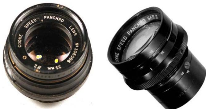
Cooke Speed Panchros for cinematography were introduced in 8 focal lengths, all f/2.0: 24, 28, 32, 35, 40, 50, 75 and 108 mm. They covered the standard format of 0.631 x 0.868 inch. These are now known as Series I. They are uncoated. (16.03 x 22.05 mm, Standard Academy film format, 27.2 mm image circle— British Patent 377,537; U.S. Patent 1,955,591-1931.)
