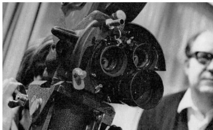
The Series III 18mm design achieved an angular field of 80 degrees, a wide relative aperture on the 18mm of f/1.7. The Series III lenses corrected for all aberrations and maintained good definition and resolution for widescreen presentation.
